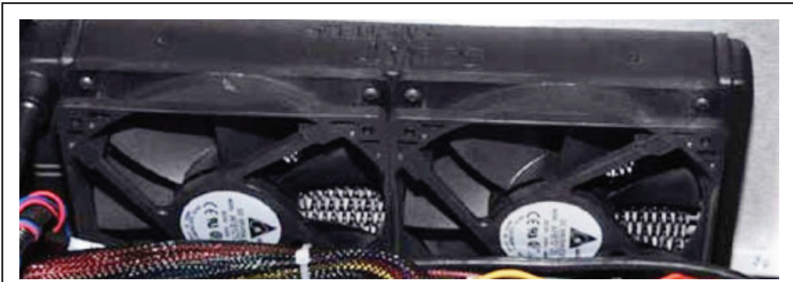
Dual intake fans pull in outside air through the front grill's radiator.
