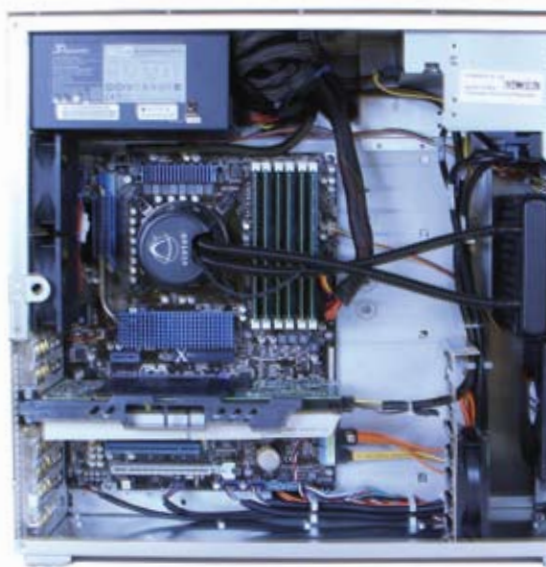
The 3DBOXX has plenty of ports, room for up to 24GB of DDR3 SDRAM, liquid cooling and six separate drives. It still manages to keep a tidy interior, in part by separating the drive bays from the rest of the components.
